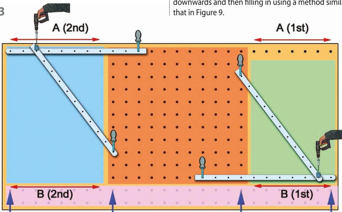
Once the top row has been extended to the left and right perform a similar operation for the lower area shown at B (1st) and B (2nd). Then complete the new columns with a single Parf Stick, held by two 3mm Pins in a similar fashion to that shown in Figure 10 which completes the blue and green area of holes.
