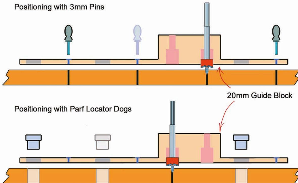
The 20mm holes are created using the 20mm Guide Block, the special 20mm cutter and either the 3mm Guide Pins or the Parf Locator Dogs.
